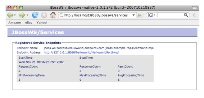
The soapUI tool can use a JBossWS "Endpoint Address" for a "New WSDL Project". Once the WSDL project is created, requests to the new web service can be simulated. A sample execution soapUI screen looks like:
