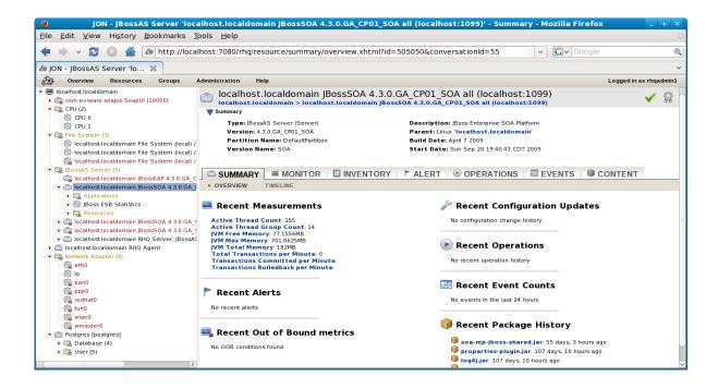
This view shows a hierarchical view of all the resources under a given platform. In this tree, one can see CPU resources, file system resources, JBoss server resources, network resources, database resource, and others. Most of these resources are folders as well and can be expanded to show more detailed child resources.
