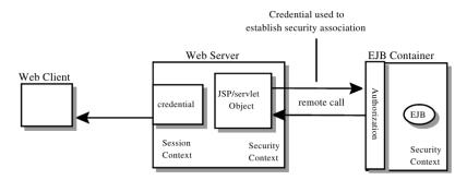
The servlet performs the remote method call to the enterprise bean, using the user's credential to establish a secure association between the servlet and the enterprise bean. The association is implemented as two related security contexts, one in the web server and one in the EJB container.
