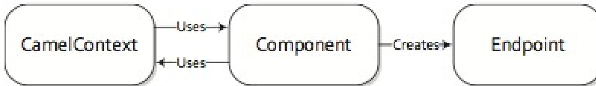
Figure 7.1 A component creates endpoints and may use the CamelContext's facilities to accomplish this.
